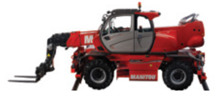
Rotation on lowered stabilisers with 1500 kg jib EN 1459
