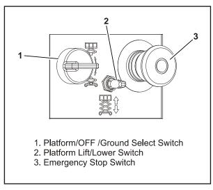
Figure 3-1. Ground Control Station
