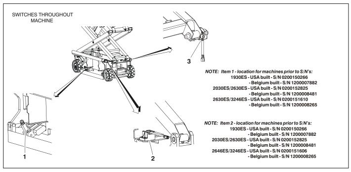
**1.** Pothole Switch - (Typical on opposite side of machine)
