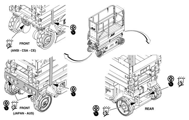
Figure 4-3. Lifting and Tie Down Diagram
