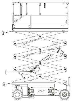
Figure 6-1. Lubrication Diagram
