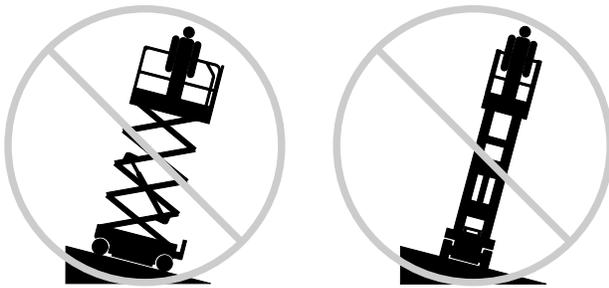
Do not depend on the tilt alarm as a level indicator. The tilt alarm sounds on the chassis only when the machine is on a slope.
