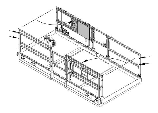
Figure 3-6. Platform End Rails - Fold Down Sequence
