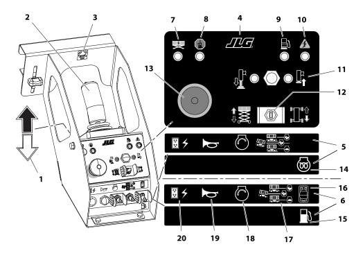
Figure 3-4. Platform Control Station
