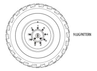
**3.** The tightening of the nuts should be done in stages. Following the recommended sequence, tighten the nuts per wheel torque chart.
