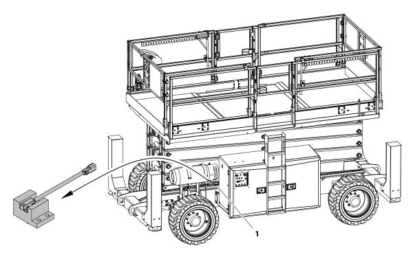
1. Scissor Arm Elevation Sensing Switch
