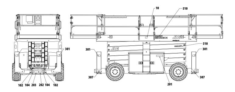
Figure 6-14. Decal Location - Sheet 2 of 4 (CE/AUS)
