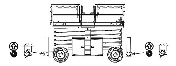
Figure 3-9. Lifting and Tie Down Chart (Sheet 2 of 2)
