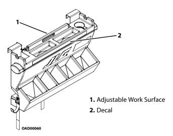
The Workstation offers an adjustable work surface and additional space for storage of tools and objects.
