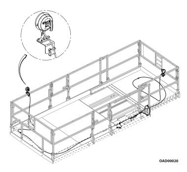
The Platform Worklights accessory consists of two 12V lights mounted to the platform railings.
