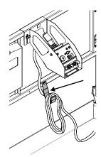
Use the hook in the platform to store excess platform cable when platform is retracted.
