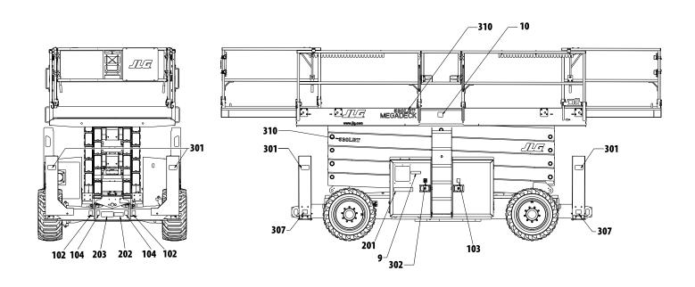
Figure 6-13. Decal Location - Sheet 1 of 4 (CE/AUS)
