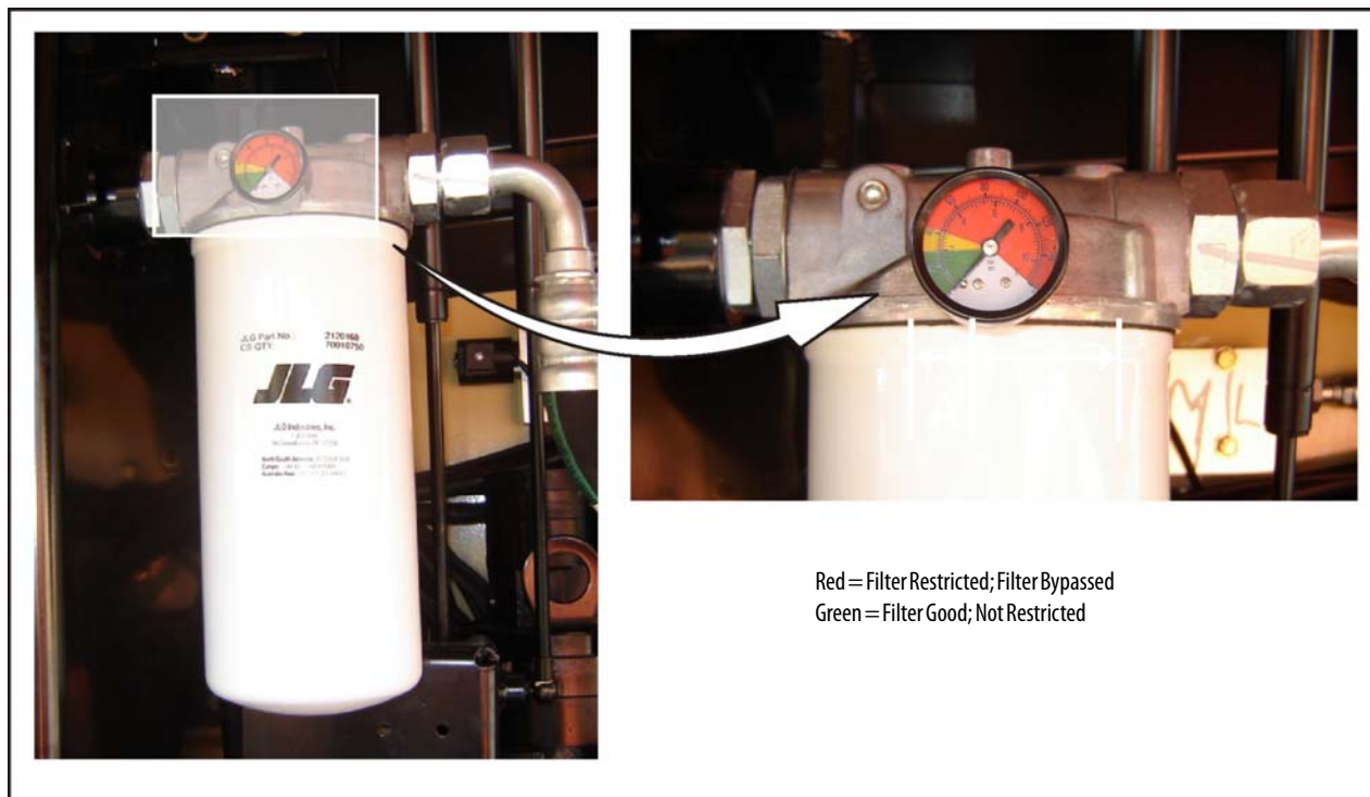
Figure 6-8. Hydraulic Return Filter Condition Indicator - S/N 139396 to Present
