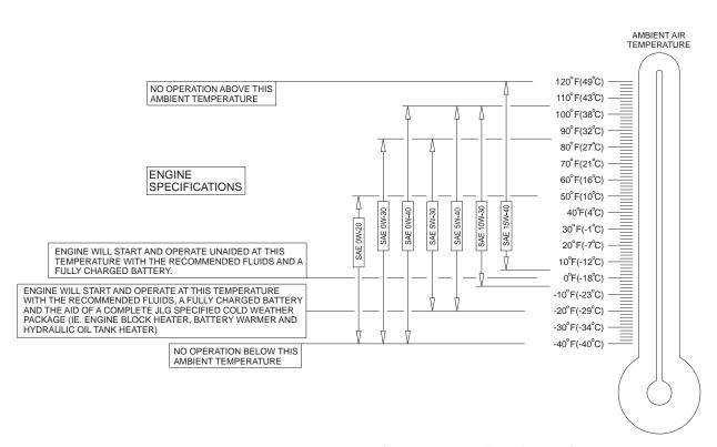
Figure 6-3. Engine Operating Temperature Specifications - Caterpillar - Sheet 1 of 2
