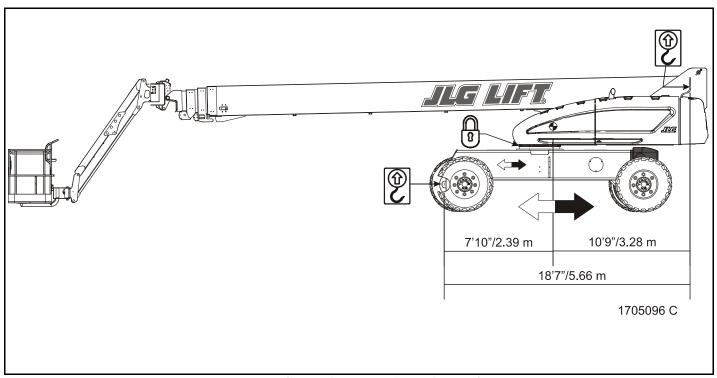
Figure 4-5. Lifting and Tie Down Chart - Sheet 1 of 2
