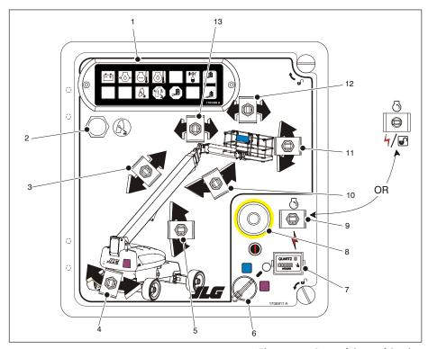
Figure 3-1. Ground Control Station
