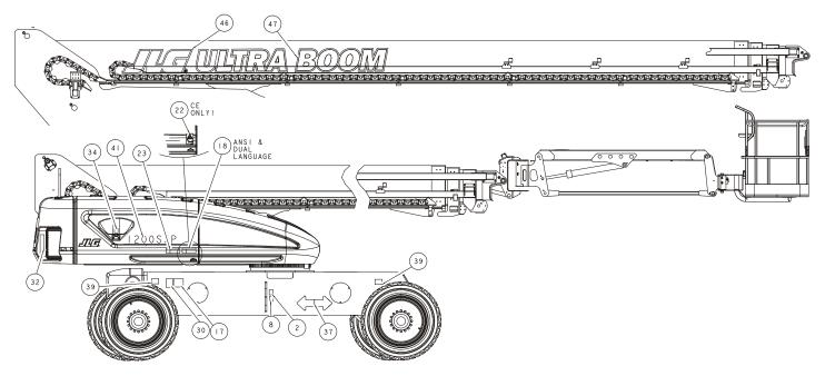
Figure 4-9. Decal Location Sheet 3 of 5
