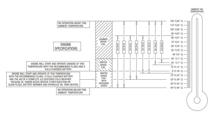
Figure 6-1. Engine Operating Temperature Specifications - Deutz - Sheet 1 of 2
