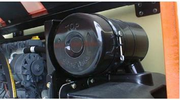
Lube Point(s) - Replaceable Element Interval - Every 6 months or 300 hours of operation or as indicated by the condition indicator
