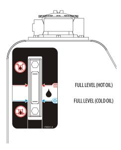
Lube Point(s) - Fill Cap Capacity - 55 gallons (208 liters) Tank Lube - HO Interval - Check level daily. Change every 2 years or 1200 hours of operation.
