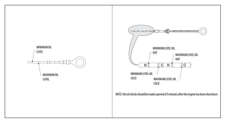
Figure 6-6. Deutz 2011 Engine Dipstick
