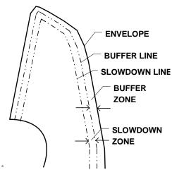
When the platform approaches the edges of the operating envelope all machine functions are slowed down automatically by the boom control system to reduce machine motions.
