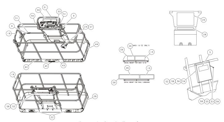
Figure 4-8. Decal Location Sheet 2 of 5
