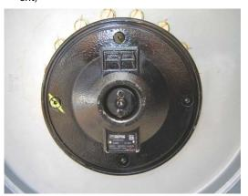
$\label{lower_loss} Lube\ Point(s) - Level/Fill\ Plug \\ Capacity - 0.5\ quarts\ (0.5\ liters) \pm 10\%$
