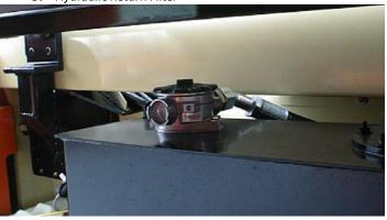
Lube Point(s) - Replaceable Element Interval - Change after first 50 hours and every 300 hours thereafter or as indicated by condition indicator
