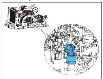
Lube Point(s) - Fill Cap/Spin-on Element
