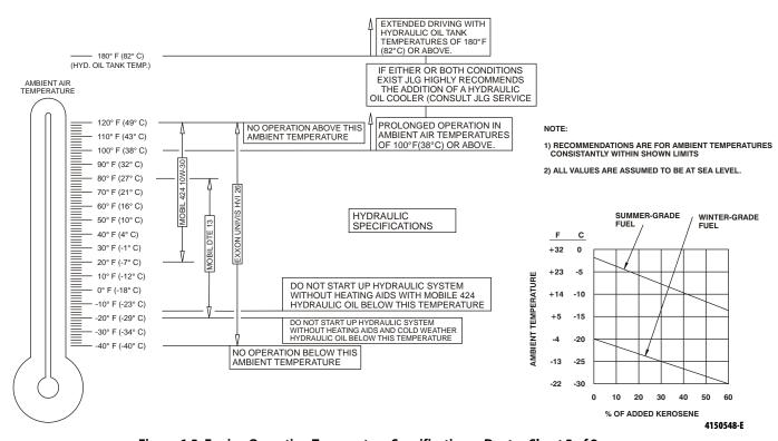
Figure 6-2. Engine Operating Temperature Specifications - Deutz - Sheet 2 of 2
