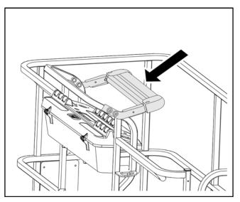
**NOTE:** If the machine is equipped with both SkyGuard and Soft Touch, functions will not reverse, only stop.
