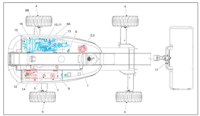
Figure 6-5. Lubrication and Maintenance Point Location
