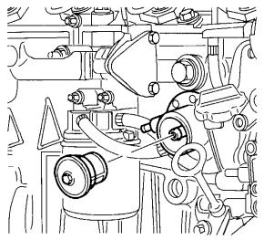
Lube Point(s) - Replaceable Element Interval - Every year or 600 hours of operation
