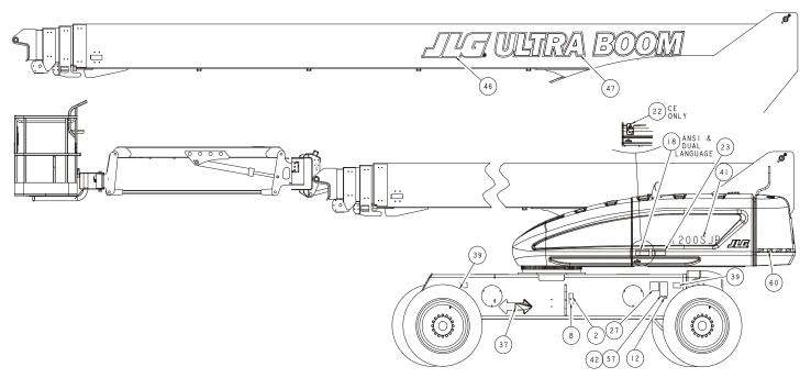
Figure 4-7. Decal Location Sheet 1 of 5
