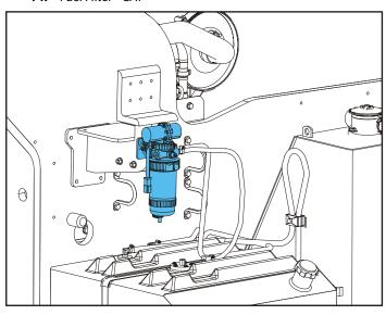
Lube Point(s) - Replaceable Element Interval - Every year or 600 hours of operation
