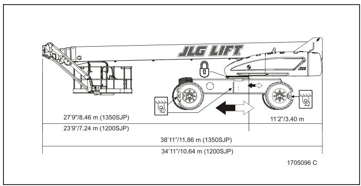
Figure 4-6. Lifting and Tie Down Chart - Sheet 2 of 2
