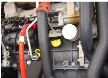
Lube Point(s) - Fill Cap/Spin-on Element Capacity - 2.4 Gallon (8.9 L)
