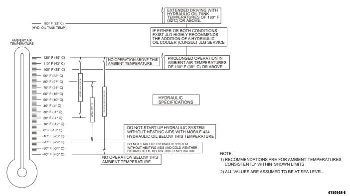
Figure 6-4. Engine Operating Temperature Specifications - Caterpillar - Sheet 2 of 2
