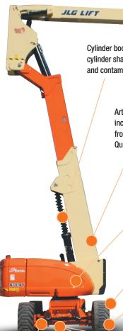
Cylinder boots protect cylinder shafts from debris and contaminants
