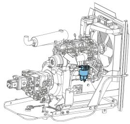
Lube Point(s) - Replaceable Element Interval - Every year or 600 hours of operation
