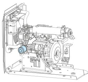
Lube Point(s) - Fill Cap/Spin-on Element Capacity - 5.4 Quarts (5.1 L) w/Filter Lube - EO
