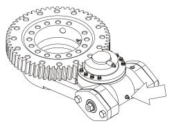
Lube Point(s) - Grease Fitting Capacity - A/R Lube - Mobil SHC 460 Interval - A/R
