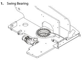
Lube Point(s) - Remote Fitting Capacity - A/R Lube - BG Interval - Every 3 months or 150 hrs of operation Comments - Apply grease and rotate in 90 degree intervals until bearing is completely lubricated 2. Swing Bearing/Worm Gear Teeth
