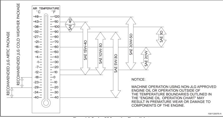
Figure 6-5. Engine Oil Operation Chart - Kubota
