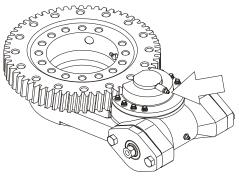
Lube Point(s) - Grease Fitting Capacity - A/R Lube - Lubriplate 930-AAA Interval - A/R
