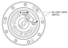
Lube Point(s) - Level/Fill Plug Capacity - 25.5 oz. (0.75 L)(1/2 Full) Lube - EPGL Interval - Check level every 3 months or 150 hrs of operation;
