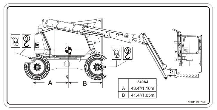
Figure 4-6. Lifting and Tie Down Chart
