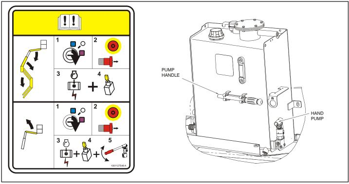
Figure 5-1. Auxiliary Descent Decal and Hand Pump
