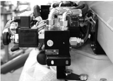
Fig. 9 Aerial part pressure relief valve
