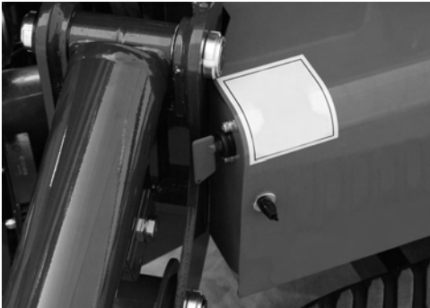
Fig. 7 Battery cut out switch thermal Engine version
