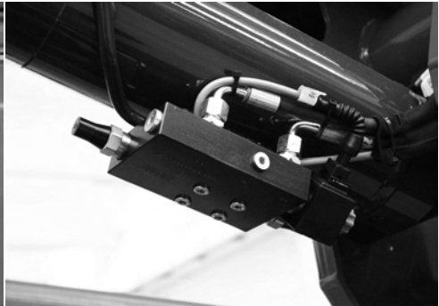
Fig. 12 Cylinder stop valves
