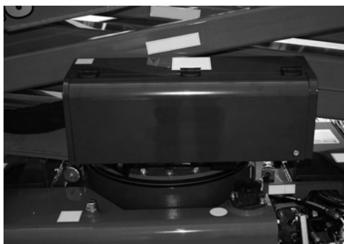
Fig. 108 Aerial part distributor protection
