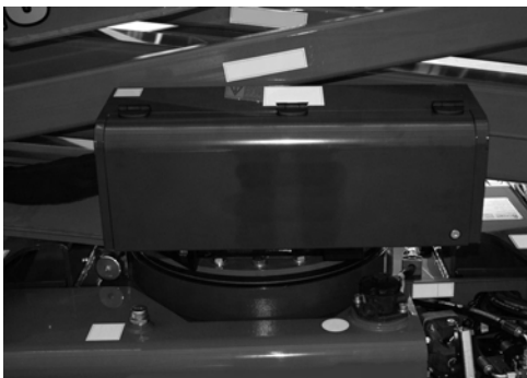
Fig. 120 Aerial part distributor protection
