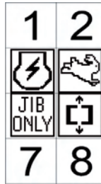
Fig. 85 Consent to use JIB during travelling
